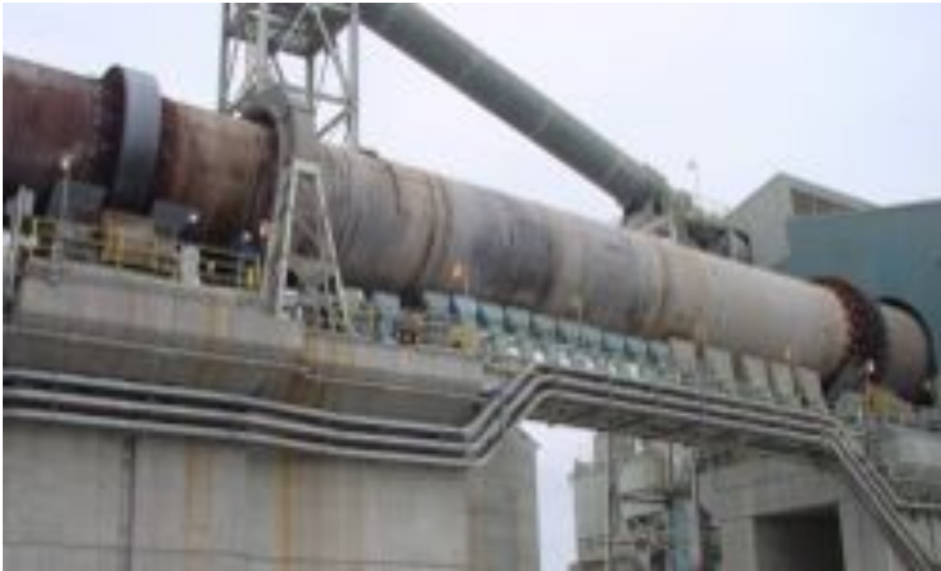
Cement kiln (Wikipedia photo). Some MWRA biosolids pellets are fuel in a MD cement kiln.
