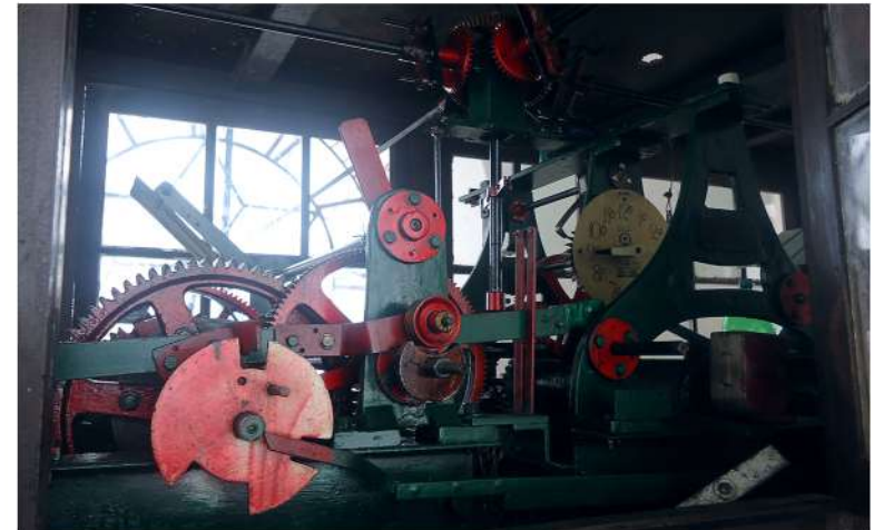
This is the original antique British clock machine that runs the KMC clock. The machine has been newly painted red and green after it was maintained by a local clock smith.
