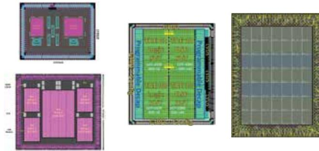
**MULTIPLE VT, 5-7 LAYERS OF METAL:** We design our IP blocks to be compatible with multiple Vt (threshold voltage) mask options and to be compatible with almost all metal stacks. eFPGA IP from FPGA chip companies will use far more metal layers so they'll typically need to redesign for your stack.
