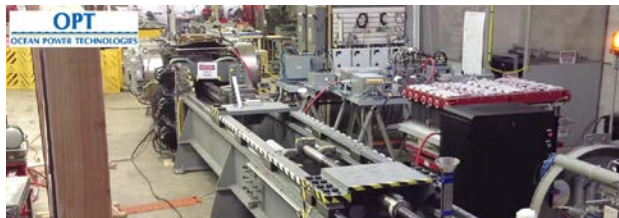
FIGURE 15: PTO ENDURANCE TEST SETUP AT OPT
