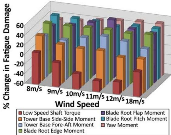
**Figure 6. Changes to Fatigue Damage Accumulation Resulting from the Addition of FlexSys Morphing Trailing Edge Technology and 10% Increase in Blade Length to 1.5MW WindPACT Turbine. Trailing Edge is 20% Chord, +/-10° Maximum Deflection, 100°/sec Deflection Rate Limit. All Damage is % Change from the Baseline Levels.**
