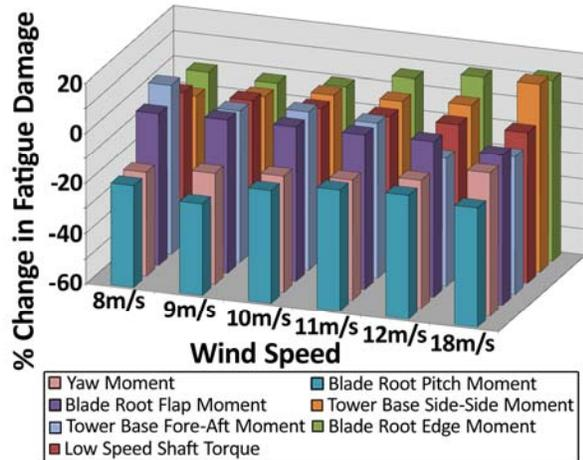
**Figure 10. Changes to Fatigue Damage Accumulation Resulting from the Addition of Conventional Flaps to 5MW NREL Offshore Turbine. Flap is 10% Chord, +/-10° Maximum Deflection, 100°/sec Deflection Rate Limit. All Damage is % Change from the Baseline Levels.**
