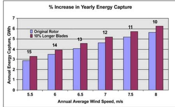
**Figure 7. Impact of 10% Growth in Blade Length on the Energy Capture of the WindPACT 1.5MW Turbine with AALC. Morphing Trailing Edge with 20% Chord Flap Length, +/-10° Maximum Deflection, 100°/sec Deflection Rate Limit.**
