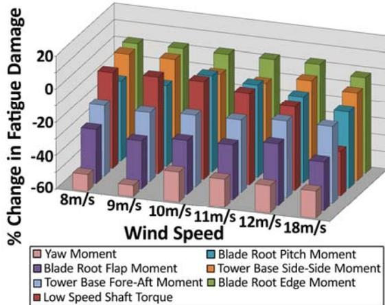
**Figure 5. Changes to Fatigue Damage Accumulation Resulting from the Addition of FlexSys Morphing Trailing Edge Technology to 1.5MW WindPACT Turbine. Trailing Edge is 20% Chord, +/-10° Maximum Deflection, 100°/sec Deflection Rate Limit. All Damage is % Change from the Baseline Levels.**
