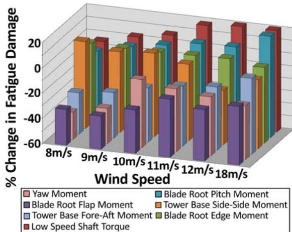
**Figure 9. Changes to Fatigue Damage Accumulation Resulting from the Addition of FlexSys Morphing Trailing Edge Technology to 5MW NREL Offshore Turbine. Trailing Edge is 20% Chord, +/-10° Maximum Deflection, 100°/sec Deflection Rate Limit. All Damage is % Change from the Baseline Levels.**
