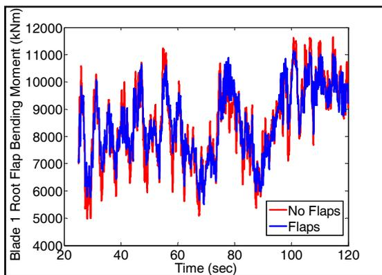
**Figure 4. Impact of Morphing Trailing Edge Technology Control on Blade Root Flap Moment of 5MW NREL Offshore Turbine at 12m/s wind speed. Trailing Edge is 20% Chord, +/- 10° Maximum Deflection, 100°/sec Deflection Rate Limit.**
