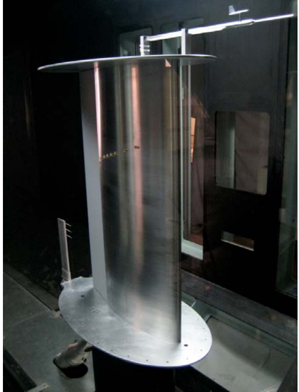
Figure 5: MAC-Wing model was tested at the Subsonic Aerodynamic Research Lab at the Wright Patterson Air Force Base (June 2006) prior to the
