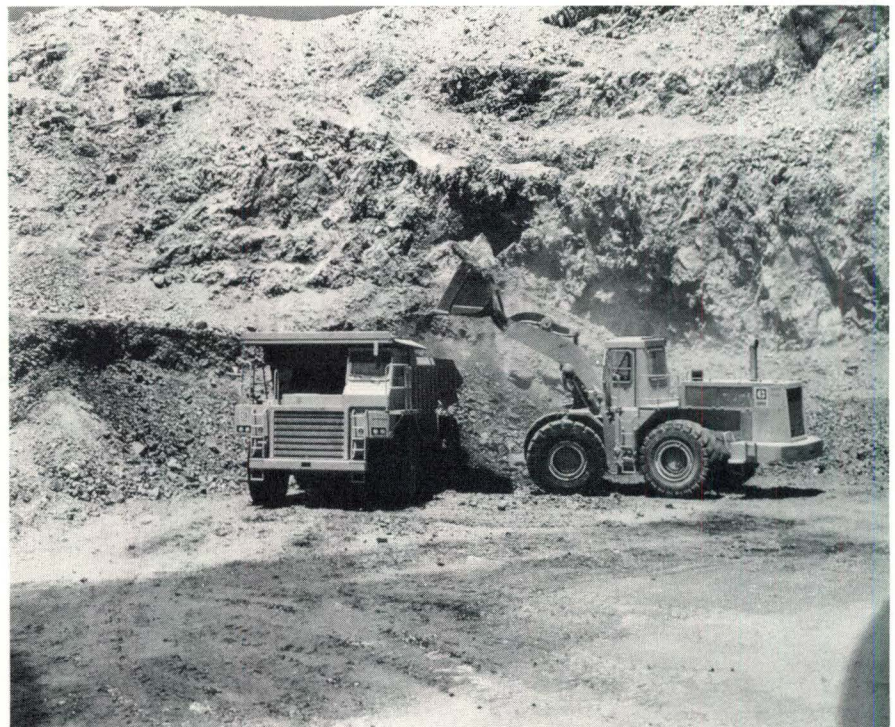
Photo 4. Mining operations are simple; a front-end loader scoops up the ore and dumps it into a truck; the truck then unloads the ore into a primary crusher. This mining method is used at the Bonny Doon shale and Bonny Doon limestone quarries.
