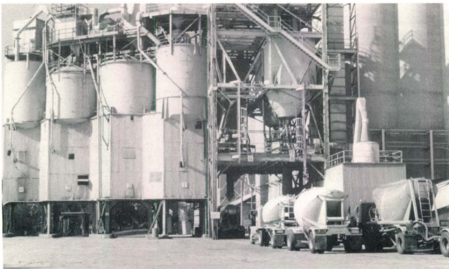
Photo 15. After the finish mill grinds the cement to powder it is conveyed to these storage silos. As needed, the cement is placed into bulk trucks (shown in photo), into handy 94 pound sacks, or into railroad cars. Most of the cement from the plant is shipped by bulk truck for customer convenience.
