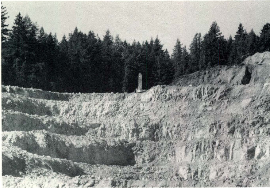
Photo 3. The Bonny Doon limestone quarry. The altered high-quality limestone is older than 136 million years and is an important natural resource. Limestone is the primary raw material used at the plant because portland cement is made from about 65 percent lime. The 40-foot-tall rig on the top bench of the quarry is used to drill the holes for blasting.
