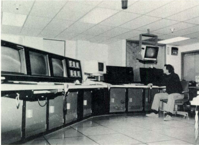
▲ Photo 8. Computer consoles in the central control room display data combined with physical outlines of the processing equipment. This allows the control room personnel to monitor production. The entire manufacturing process except for quarry and shipping operations is fully automated and under continuous computer control. When a variation anywhere in the manufacturing process requires an adjustment, corrections are automatically signaled from the central control room.
