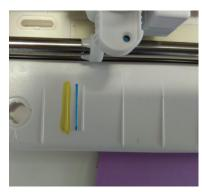
Mount printed or bare cardstock onto the Silhouette Portrait 2 cut mat by placing the project onto the sticky surface so that the top-left corner is aligned with the marks on the cut mat labeled 8½" x 11" (see image above). Feed the cut mat into the Silhouette Portrait2 by aligning the left edge of the cardstock (not the cut mat) to the center line of the group of short lines on the left side of the feed area. Press the **Up Arrow** button on the Silhouette Portrait 2.
