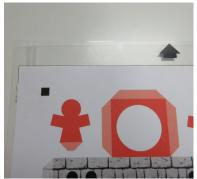
Mount printed or bare cardstock onto the Silhouette Portrait cut mat by placing the project onto the sticky surface so that the top-left corner of the paper is aligned with the marks on the cut mat labeled 81/2" x 11". Feed the cut mat into the Silhouette Portrait by aligning the left edge of the cardstock (not the cut mat) to the center line of the group of short lines on the left side of the feed area. Press the **Load Cut Mat** button on the Silhouette Portrait.
