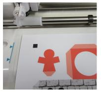
Click **Send to Cutter** to begin fabricating your project. The Silhouette digital fabricator will scan and detect the registration marks if the option is selected, and proceed to cut the paper.
