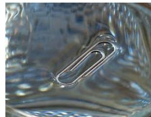
**Surface Tension** is the tension of the surface film caused by the attraction of the particles in the surface layer.
