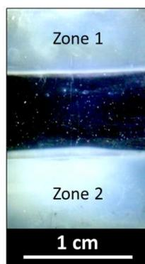
**Figure S8.** Photograph of the deposited metal-organic framework coatings HKUST-1 + HPA (Zone 1) and HKUST-1 (Zone 2).
