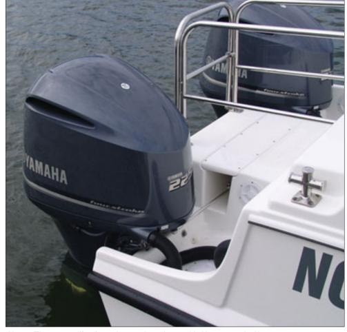
Above: The new tooling in and around the transom and outboard wells is beautifully done - note the 'tunnel" for the steering tie bar, the walk-thru transom door and fold-down ladder.
