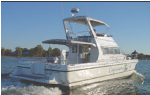
This is impressive - the latest 285 hp Volvo Duo Prop sterndrives, pushing nearly 9 tonnes of 4400 NoosaCat to 30 knot performance, and very laid-back cruise around 24-25 knots. Installation standard is superb.
