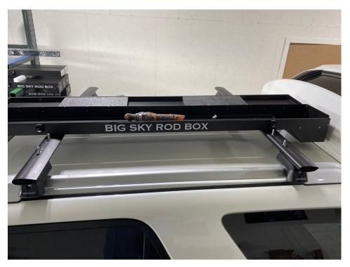
7. Lift the box onto the t-bolts. This is often easier with two people. Use the supplied t-bolts, washers, and <u>nyloc nuts</u> to secure the box. (NOTE: Nuts and washers should go on the inside of the box.)
