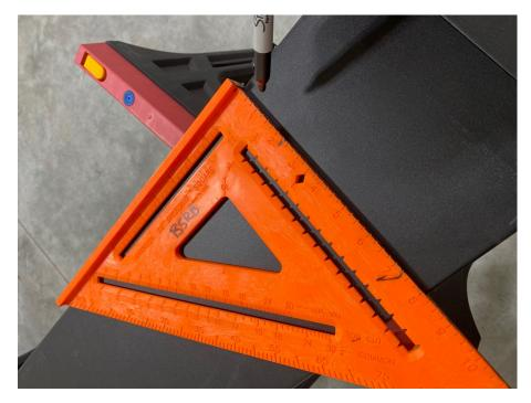
5. Drill four holes in the bottom of the box. Two for the front bar and two for the rear. It's good to oversize the holes to make the u-bolts easier to insert. (HINT: Position the holes 2 ¼ inches in from the edge of the box to ensure the bolt heads will be under the thickest part of the foam rod dividers.)
