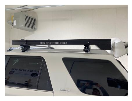
2. Once positioned, mark the center of t-slot on the side of the rod box for both the front and back cross bars.
