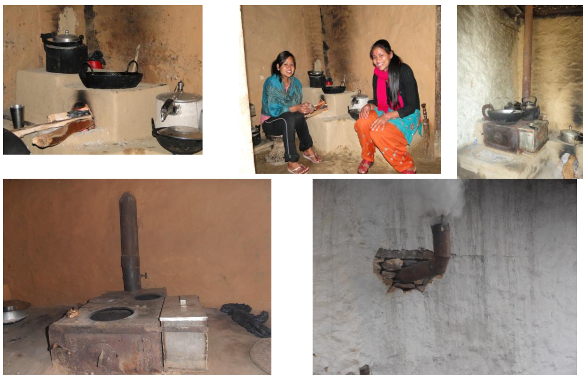
Figure 6: Top Left: A two pot clay stove in action; Top centre: Sociable and easy to use; Top Right and Bottom Left: Full metallic stove installed; Bottom Right: the proper place for kitchen smoke
