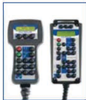
Full function remote control 4-axis or 6-axis with welding program selection
