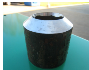
37.5 deg bevel on 2.500 x 0.500 inch wall tubing cycle time 15 seconds
