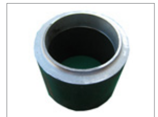
J-bevel on 2.500 x 0.312 inch wall tubing cycle time under 20 seconds
