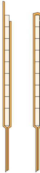
*Note coil placement in foldover tab per most OEM designs. The top coil sits only halfway up the short side of the riser, leaving little material on the long side to bend.*
