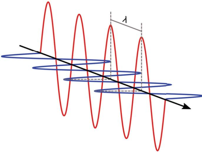
**Figure 1** | Electromagnetic excitations are made up of a wave of electrical energy (red) together with wave of magnetic energy (blue). The two propagate in the same direction, but are perpendicular to each other. The wavelength, usually represented by the symbol  $\lambda$ , is the distance between adjacent peaks of the two constituent waves and is inversely proportional to the frequency; that is, the number of undulations (or oscillations) up and down per second.
