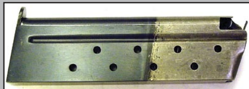
Two-toned, pinned-base magazine. The “slot” at the top was added at about SN 10000 to aid feed reliability.
