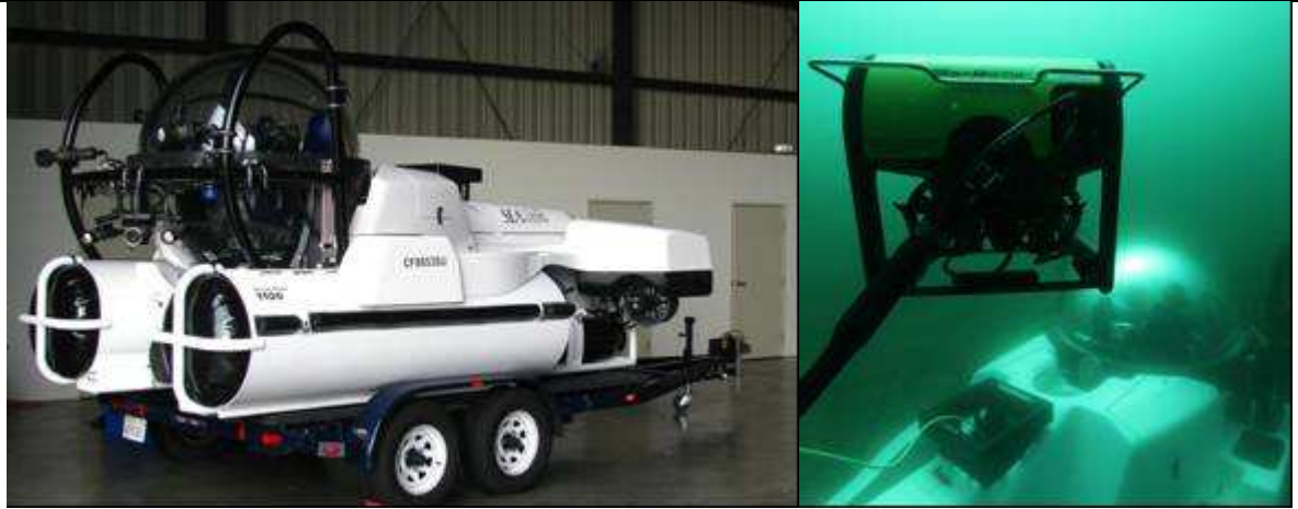
SEAmagine No. 9 Submersible ABS Classed to 1100 ft with Fly-Out ROV system & HD Cam
