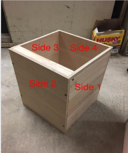
Figure 1: The test box with and without the front temporary wall. Inner dimensions are 12"x12"x16"
