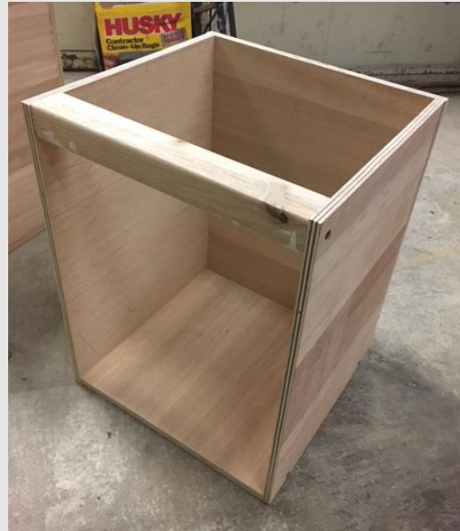
Figure 1: The test box with and without the front temporary wall. Inner dimensions are 12"x12"x16"
