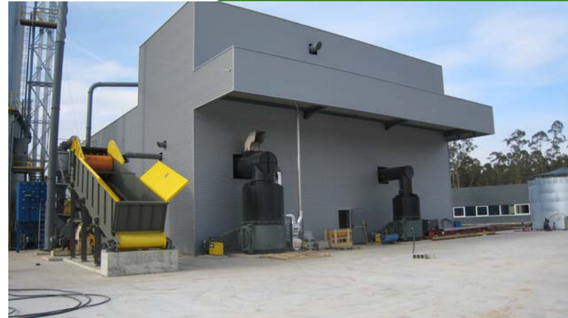
CYCLOCLEAN SOLID BIOMASS BURNER FOR HEATING Z8 BIO- MASS DRYER & TORREFACTION REACTOR
