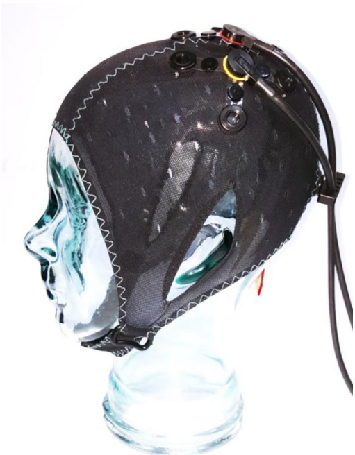
fig 1. The NIRx NIRScap with integrated TMS optodes. The optodes are completely compatible with TMS stimulation. Their low profile allows for very close placement of the TMS coil.
