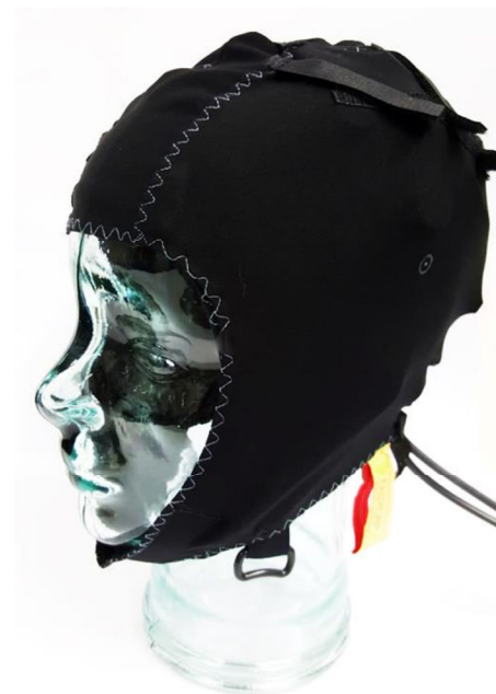
fig 2. The NIRx TMS compatible overcap, placed over the NIRScap. The retaining cap stabilizes the setup making it more robust to TMS coil contact artifacts and motion artifacts in general.
