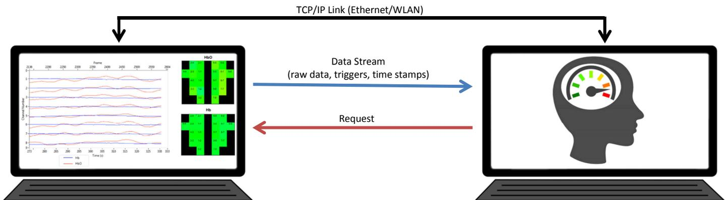
The real-time data stream, as depicted above, can be easily achieved with the NIRx Software Development Kit (SDK), which provides a dynamic library that allows the user to communicate with the acquisition software. \*Users without programming knowledge may also easily benefit from SDK with the several examples available.
