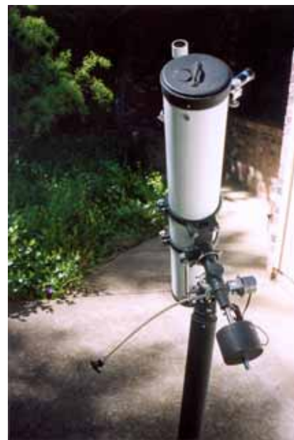
Figure 2. The author's deluxe 4-inch f/10 (1000mm focal length) equatorial reflector telescope.
