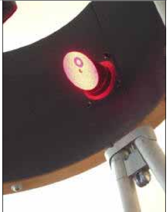
This view is looking up toward the Blug inserted into the inside end of the focuser of an Obsession telescope. Note the shadow of the primary mirror's center donut. Photo from Howie Glatter's website: http://www.greatredspot.com/collimator.htm .
