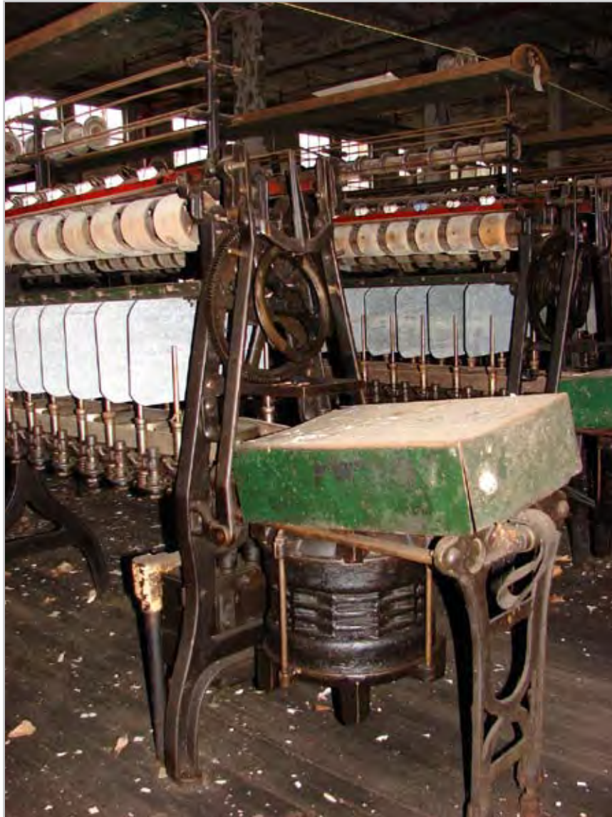
Plate 5.16. A silk throwing machine with electric motor, 2007. [Klotz Throwing Mill, near Cumberland, Maryland]. Compact motors allowed mill operators greater flexibility in locating machines. Electric power had been applied to machines at the Todd Mill prior to 1915. The other mills at the ATP site fully electrified after the S.U.M. power plant opened in 1915. Electric operations also allowed landlords of the ATP's mills the flexibility of renting out space to tenants without having to regulate central direct-drive power systems. By 1915, all of the ATP's mills were tenant mills. Source: Patrick J. Harshbarger, 2009.
