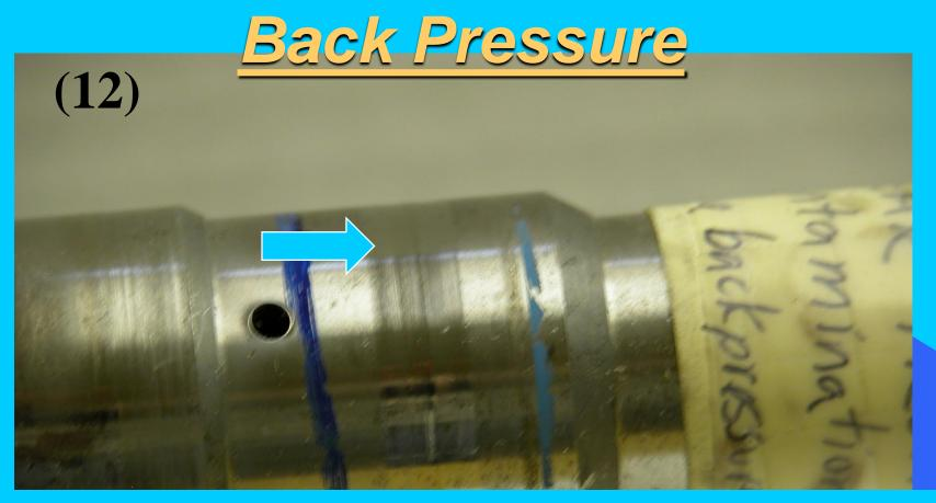
Dirt and back pressure will cause grooves in seal area on motors
