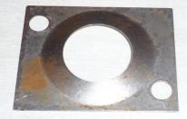
Plate bowed out from pressure pushing O ring out of bore
