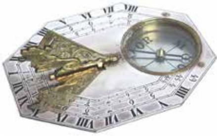
Fig. 16 Butterfield Dial by Bizot using a Lion as the Gnomon supporter:
