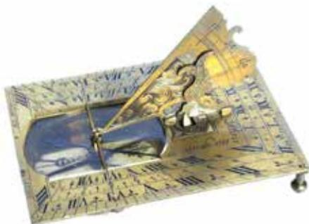
Fig. 18 Dial by Le Maire with its Gnomon supported above the Compass.
