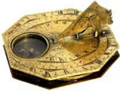
Fig. 25 Butterfield Dial situated on top of an Equatorial Dial.
