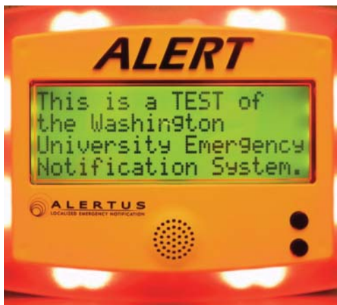
The Alert Beacon, a wall-mounted audible visual notification appliance, is one of several devices that Washington University in St. Louis uses to notify faculty, staff, and students in the event of a threat.
