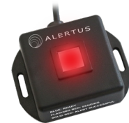
USB Panic Buttons enable one-touch, immediate incident reporting or system activation
