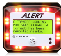
The wall-mounted Alertus Alert Beacon® sounds, flashes, and displays an alert message in the event of an emergency
