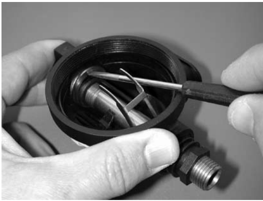
Fig. 1 – Removal of Retaining Clip
