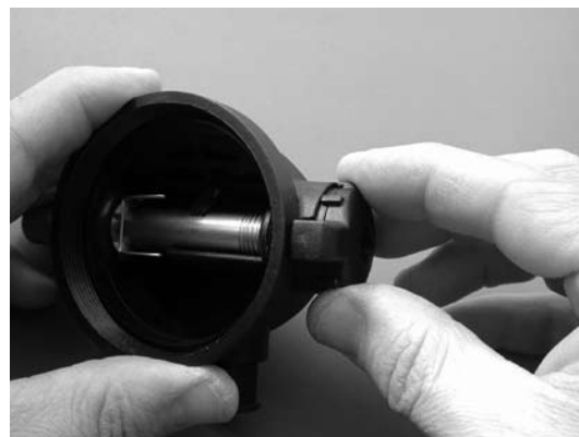
Fig. 19 – Correct Position of Venturi Switch
