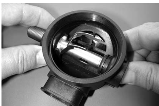
Fig. 15 – Valve Assembly Completely Installed
