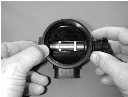
Fig. 2 – Removal of Valve Assembly
