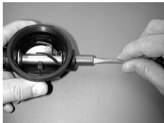
Fig. 20 – Preliminary Orifice Setting
