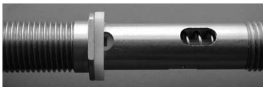
Fig. 12 – Poppet Correctly Installed
