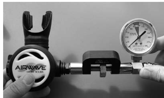
Fig. 21 – Inline Adjustment Tool w/ IP Gauge
