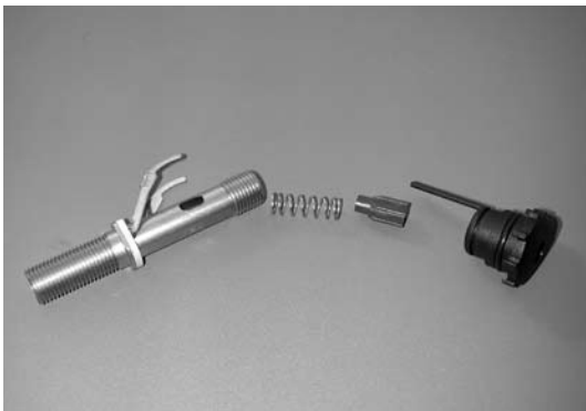
Fig. 3 – Removal of Venturi Deflector
