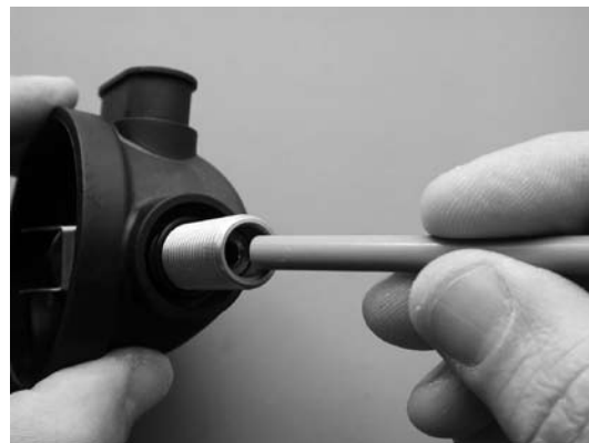
Fig. 17 – Installation of Orifice
