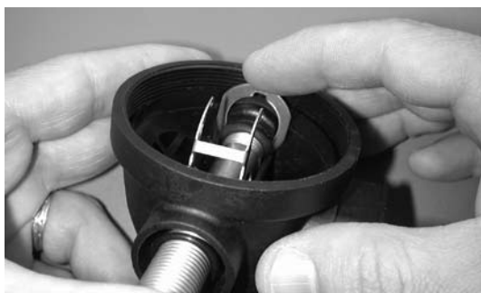
Fig. 16 – Installing Retaining Clip
