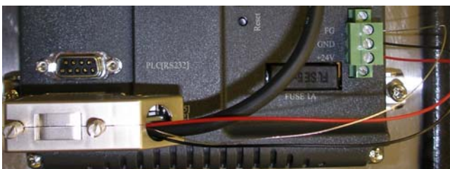
Power wires from Female DB9 connector to terminal strip on Touch Screen
