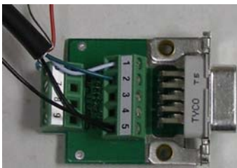
Connections in Female DB9 connector on Touch Screen
