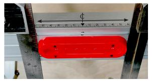
A mortise and tenon <sup>1</sup>/<sub>8</sub>" larger or smaller than the sizes shown on the chart can be made using one circle end-piece and one triangle end-piece. The centering hole will be off by <sup>1</sup>/<sub>8</sub>" when using the templates this way, so use the measuring method described above to center them.
