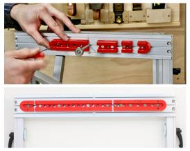
Several segments can be combined for large arrays. In this case the combination makes a 4" mortise and tenon, 3%" thick.
