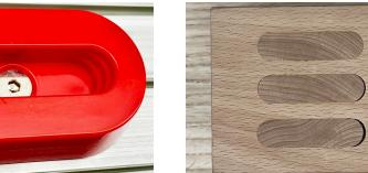
The three steps in the ends of the mortise slot allow three widths of mortise. Use the lowest step when you need a perfect fit side-to-side such as for through-mortise and tenon. Use the second or third step if you prefer a little side-to-side adjustability, which can sometimes be helpful during glue-up. Using the third step allows room to wedge the tenon.
