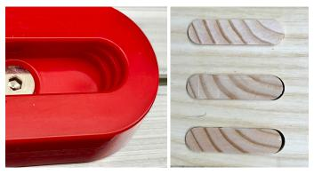
tise slightly wider than the tenon, the second or third step can be used. This additional room side-to-side is sometimes useful for adjustability during glue-up or for wedging the tenon to strengthen and visually enhance the joinery. M&T templates are supplied in two styles, Standard and Segmented, and they use different sizing schemes.
