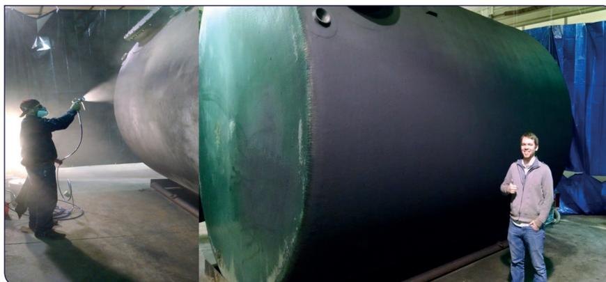
Fig. 1: Applying NEETcoat® with an airless sprayer (left); glass fibre tank prototype with NEETcoat® for static dissipation protection (right)
