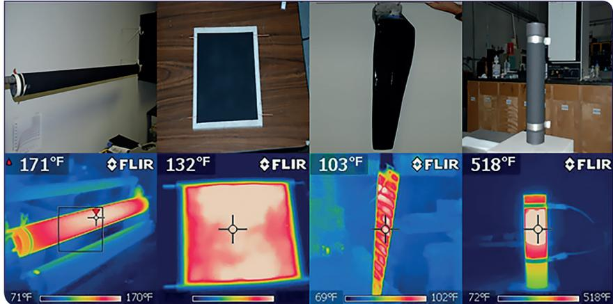
Fig. 3: Examples of materials heated with NEETcoat®, from left to right: 1) 76-mm OD carbon steel pipe, 2) cement board panel, 3) epoxy composite wind blade, 4) steel pipe prototype of High Temp NEETcoat®
