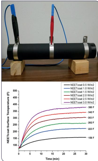
Fig. 2: NEETcoat® applied to pipe (up); graph of NEETcoat® surface temperature compared to applied power density (down)
