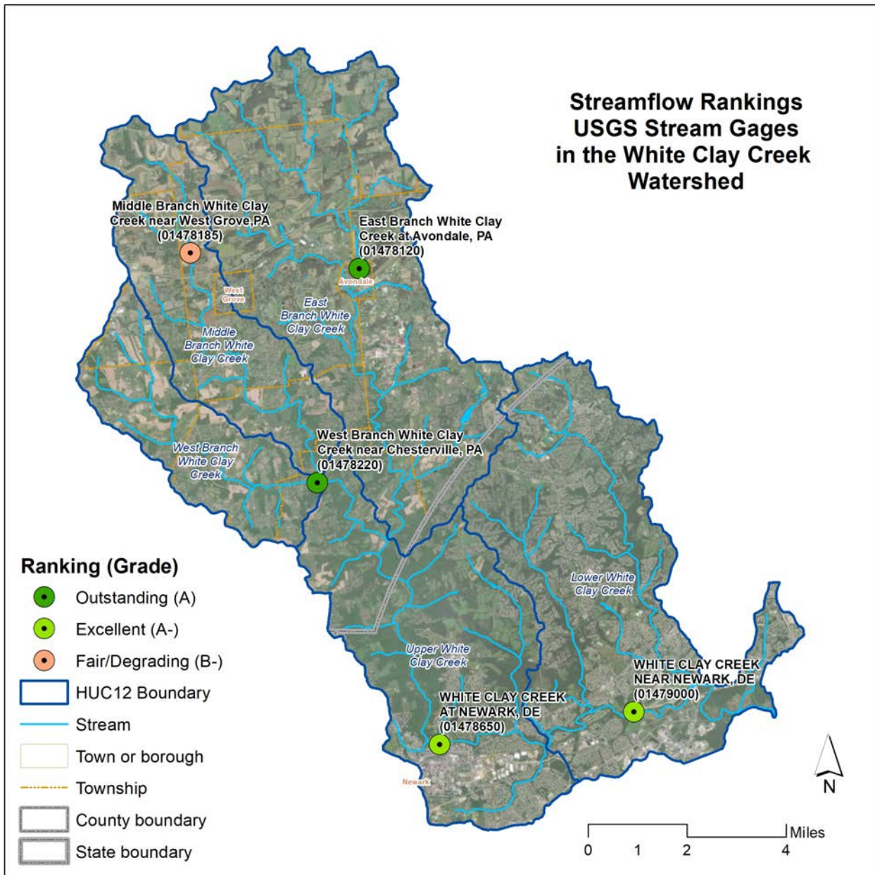
Figure 29. Gaging station and grades based on flow
