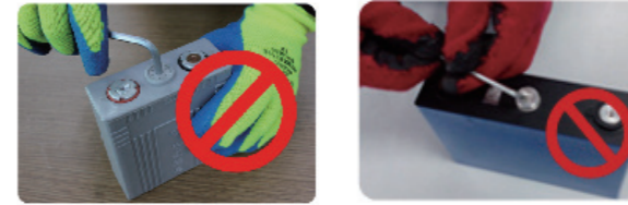
Damaging the battery safety valve is forbidden without permission.
