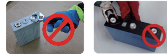
Screwing the battery terminal is forbidden without permission.
