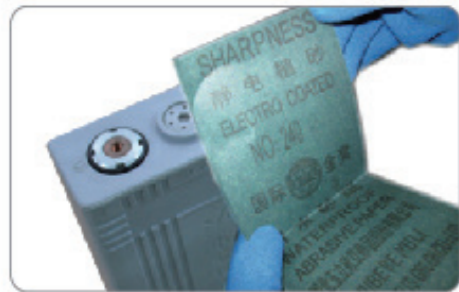
Battery terminal pole sanding
