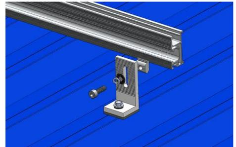
Once you have securely fixed all 4 brackets you can now fix the top and bottom rail to the brackets with the Allen key head screw, washers and nut modules provided. Tighten Allen key screws nice and firm. See below...
