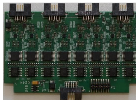
Fig. 2, eAMP-I PCB board (top view)
