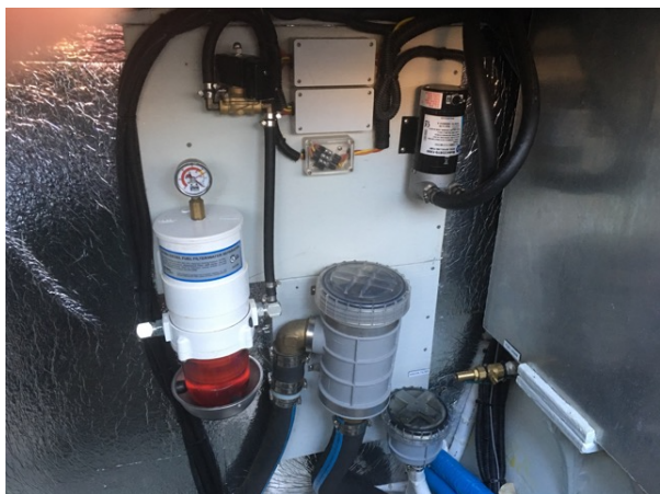
Port Engine compartment: Racor filter and Gauge, Large engine strainer, Air conditioner strainer
