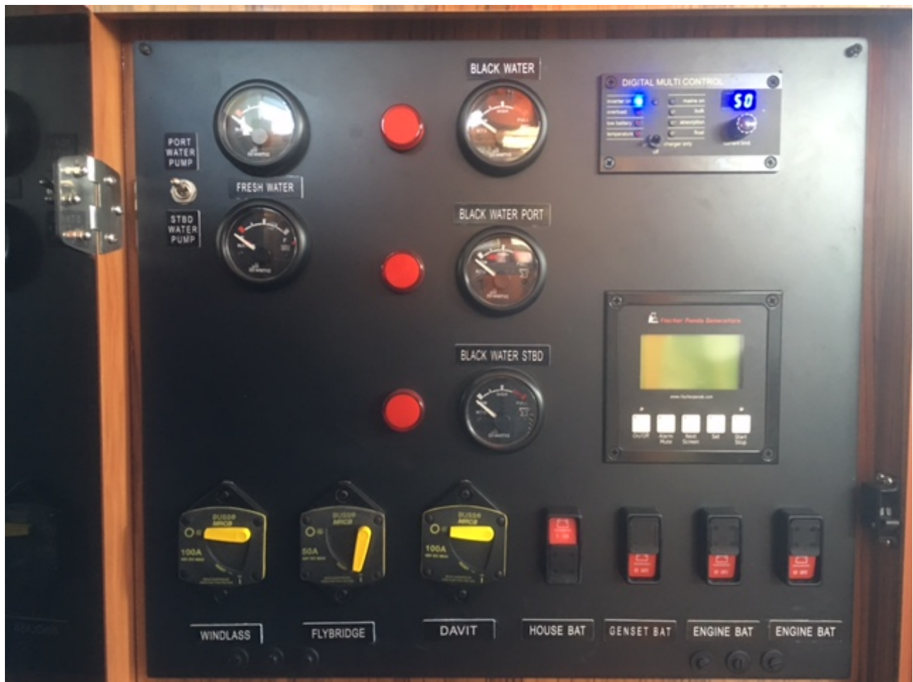
In the photo above the FLYBRIDGE and HOUSE BAT switches are in ON position. All others are OFF.
