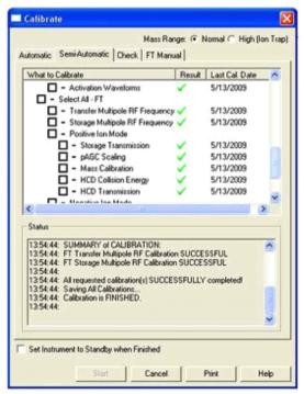
Usually, you do not need to perform a complete ion trap calibration or an FT ion transmission calibration unless the hardware is modified in some way. However, it is necessary to repeat the electron multiplier calibration monthly and the FT mass calibration weekly. To perform an FT calibration, the ion trap has to be successfully calibrated before. The calibration masses and all experimental parameters like target values, scan ranges, resolution settings, etc. are set automatically.
