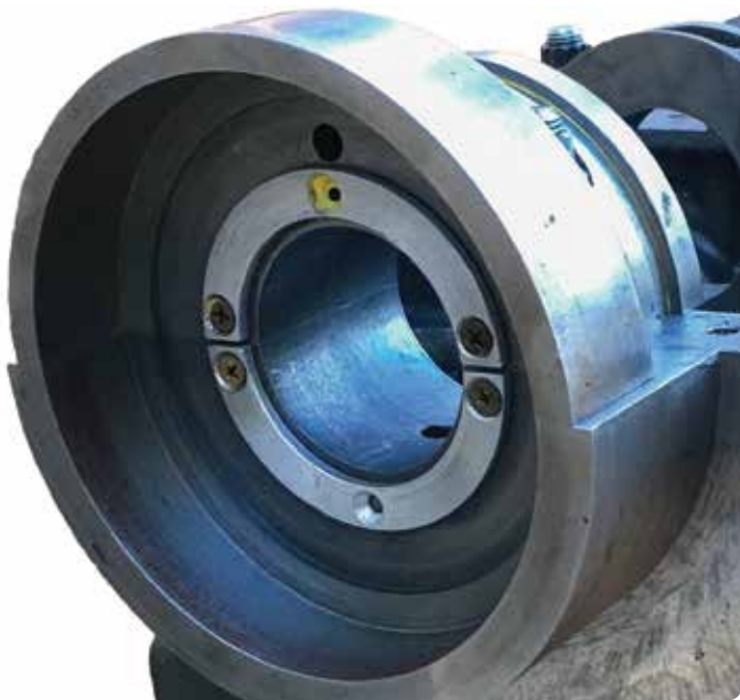
For aircraft use, the rear main bearing, which is in front on an airplane, is easily reassembled to be pulled on rather than pushed, as it is in a car.
