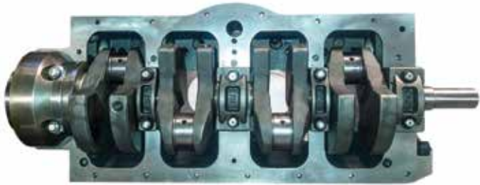
The dynamically balanced crankshaft is installed. It has five journals (as opposed to the original three) and full insert bearings rather than Babbitt bearings so it is a far cry from the original.
