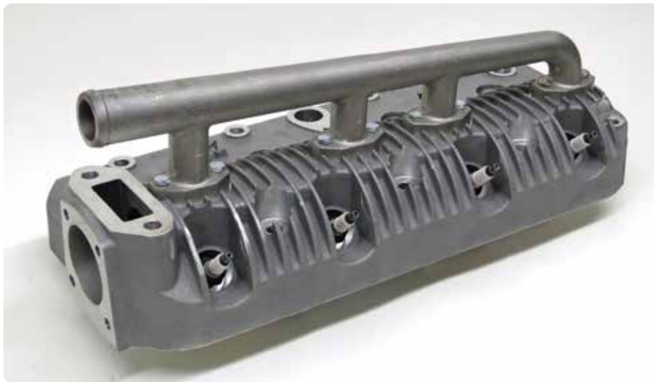
A number of aluminum, high-compression heads are available from various sources. The 6.5-to-1 compression ratio, two-plug-per-cylinder Rocket 428 head, shown here with the optional racing cooling tube, is available from SecretsOfSpeed.com .
