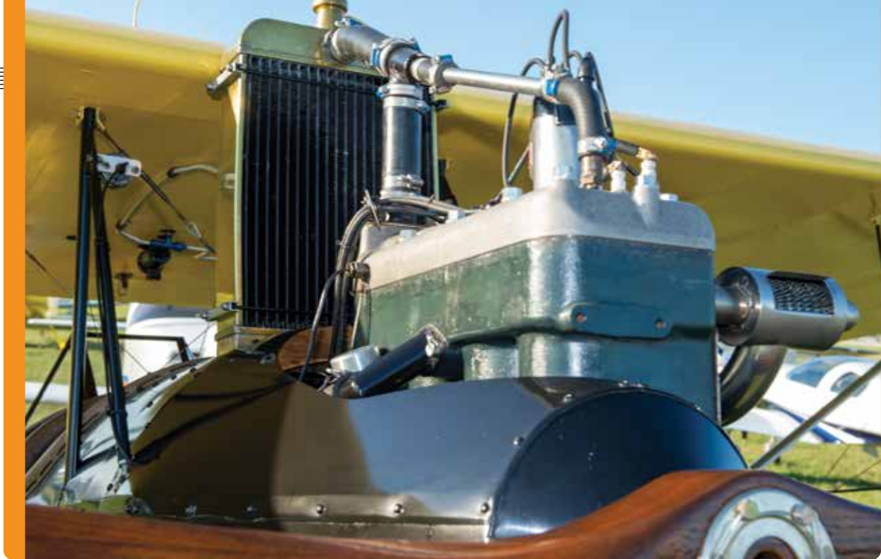
The 90-year-old Model A engine is usually seen dragging a Pietenpol around (Dan Helsper's award-winner), but other designs used it, too. The Burtz Model A block brings new-age technology to the old war horse.
