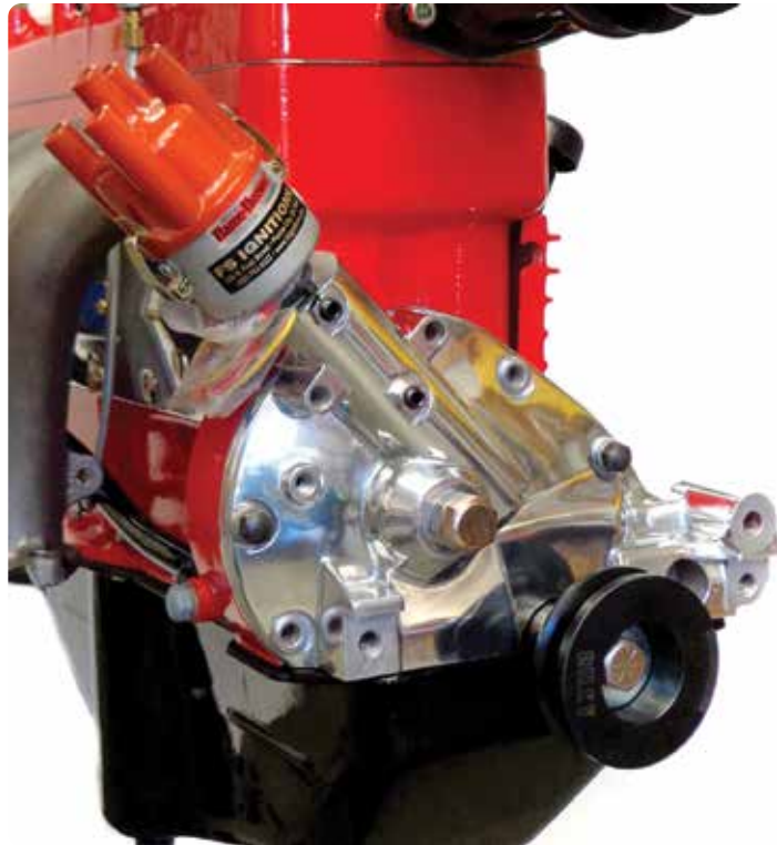
Old WICO mags that drop right in the original distributor hole in the head can be found on eBay and paired with a rear-mounted mag to give dual mags. The Secrets of Speed front (rear on aircraft) ignition drive mounts VW distributors or magnetos.
