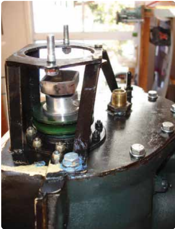
Bernard Pietenpol designed a super-simple DIY magneto mount to be hung on the front (aircraft rear) of the engine and is belt driven from the crank pulley.
