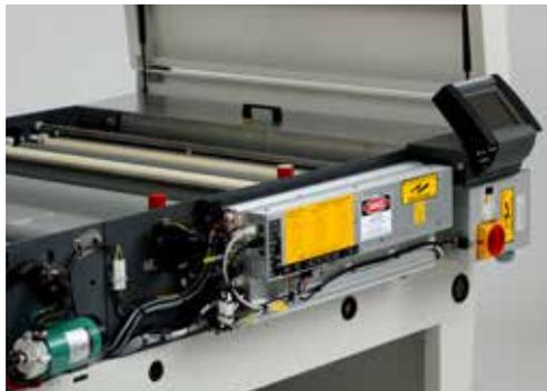
Easy-lift top covers provide good access to the inside of the processor. The electronics are conveniently located on the side of the processor.
