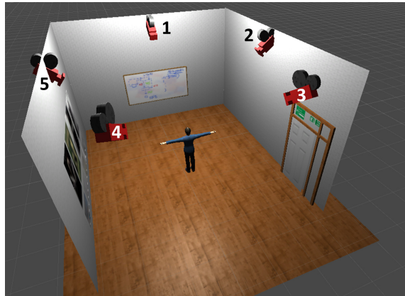
Figure 1. A seminar room simulated in Unity3D © with 5 ceiling-mounted cameras in a pentagonal arrangement (cameras are numbered accordingly). A single omni-directional light source was used to illuminate the entire room. For visualization, this light source has higher intensity than shown in Figs. 2 and 3.
