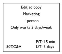
In addition to calculating the key metrics for each process block, you need to calculate the summary metrics for the value stream. Add the process time and lead time for each process block to get the total P/T and L/T. Multiply the %C&A for each process block to get the total for the value stream. Run the time line and summary metrics below the map:
