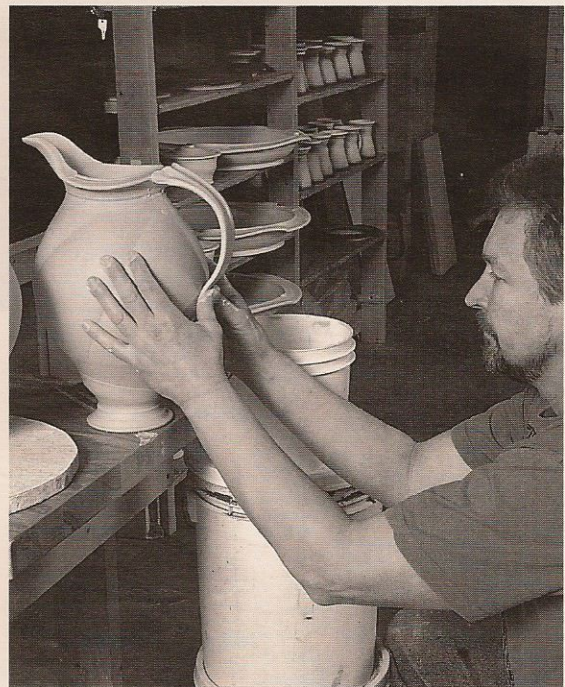
Figure 13. I use a simple sweeping motion with my thumbs to join and finish the tail end of the handle. After finishing the handle, it is a good idea to cover the pot with plastic overnight, so the water content will even out and lessen the chance for cracking.
