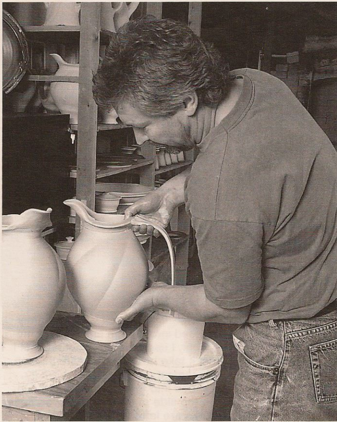
Figure 11. I then set the pot upright on the edge of a table, gently supporting the curve of the handle.
