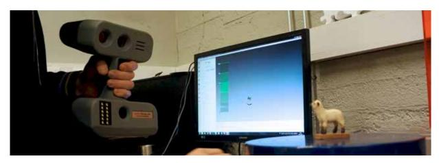
**ABOVE:** ATTEMPTING TO SCAN DOLLY USING AN ARTEC MHT SCANNER
