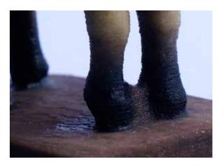
ABOVE: DETAIL SHOT SHOWING DOLLY'S LEGS FUSING IN THE 2ND GENERATION. RIGHT: FIFTH AND FINAL GENERATION.
