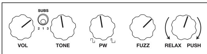
**RELAX/PUSH:** This knob introduces source impedance to the signal going into the Mastotron™. When fully up, the signal goes in raw... when turned down, source impedance is added as needed to "soften" the input for active pickups.
