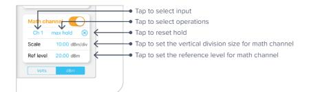
Four operations are currently supported by Moku:Lab Spectrum Analyzer: +, ×, min hold and max hold.
