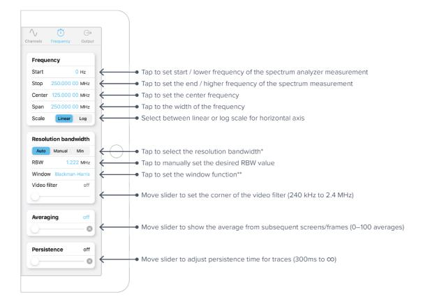
Note that [Start, Stop] and [Center, Span] in the frequency panel are equivalent representations of the measured frequency range. The Moku:Lab will automatically update the other pair if one is changed.
